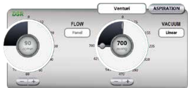
VENTURI/ROTARY VANE PUMP Vacuum: up to 700 mmHg
